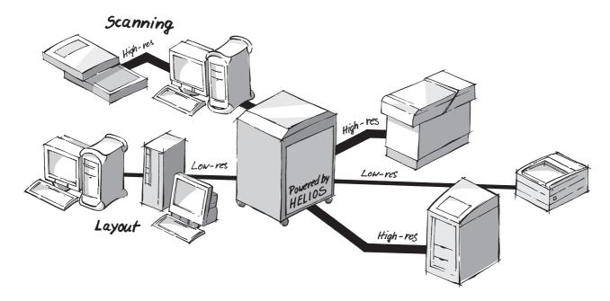
HELIOS ImageServer UB2 is a server-based image conversion, color transfor-mation and OPI image replacement solution, with integrated process and workflow automation. All major image formats and color spaces as well as XMP, EXIF, clipping path and ICC meta data are supported. Tasks can be automated via "hot folders", CLI tools, and OPI image repurposing. It is designed to shift very CPU-intensive image processing tasks from desktops to servers.
