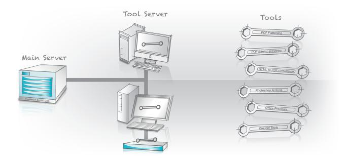
**Tool Server G8** allows applications running on network clients to be automated and remotely used by the HELIOS server. Many applications and technologies are only available on a specific platform. Tool Server makes these required applications and technologies available to your HELIOS server, as a standalone process, or for integration into server workflows.
