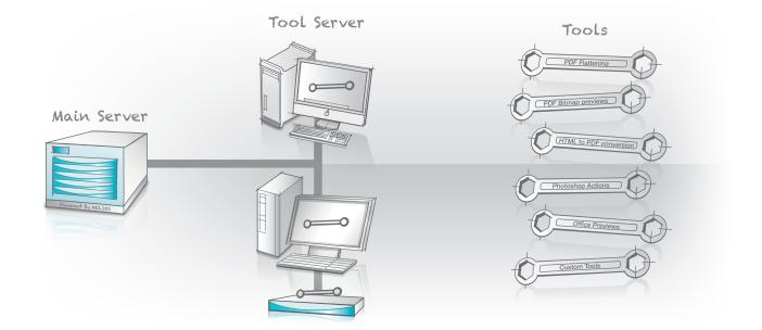
**Tool Server** allows applications running on network clients to be automated and remotely used by the HELIOS server. Many applications and technologies are only available on a specific platform. Tool Server makes these required applications and technologies available to your HELIOS server, as a standalone process, or for integration into server workflows.
