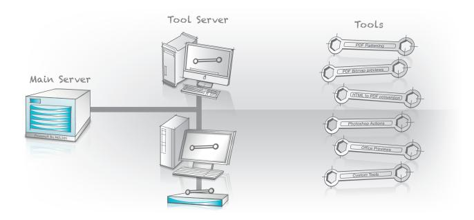
Tool Server G8 allows applications running on network clients to be automated and remotely used by the HELIOS server. Many applications and technologies are only available on a specific platform. Tool Server makes these required applications and technologies available to your HELIOS server, as a standalone process, or for integration into server workflows.
