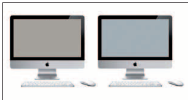
Figure 2. A representation of a display set at D50 (5000K) and D65 (6500K).
